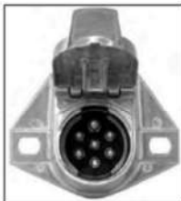
Standard seven-pin connectors for primary electrical lines include all-female terminals in the plug and all-male terminals in the receptacle.
