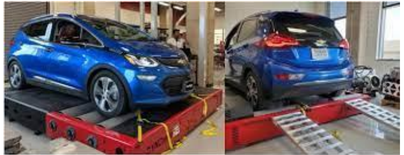
Figure 1. Chassis dyno with EV under test.
